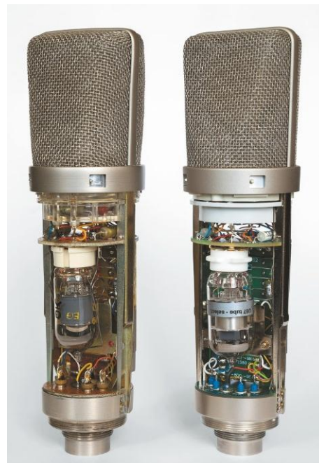
There are hardly any changes to the backside, either. The reissue has no mounting bracket for the tube because, as was found out later, it has no function: The socket is so tight that the tube won't move, with or without a bracket.
