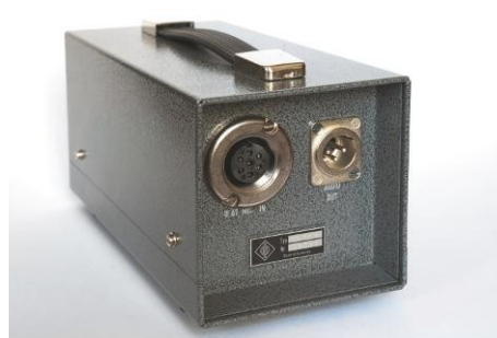
The higher filament current demands of newer tubes and stricter safety regulations necessitated a new power supply.
