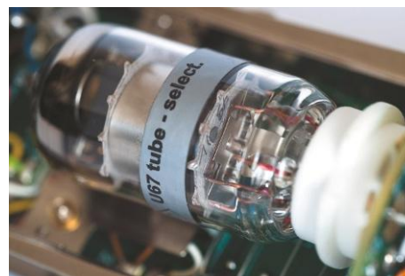
The U 67 reissue uses a current production EF86 type tube without a manufacturer stamp. Each tube is meticulously tested and selected by Neumann.
