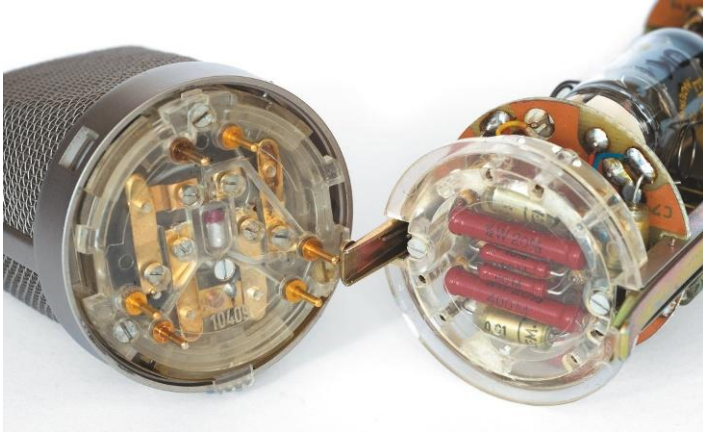
The bottom of the detachable capsule head and its counterpart were made of acrylic glass, which tends to crumble with age. The U 67 from Echoschall is still immaculate, though.
