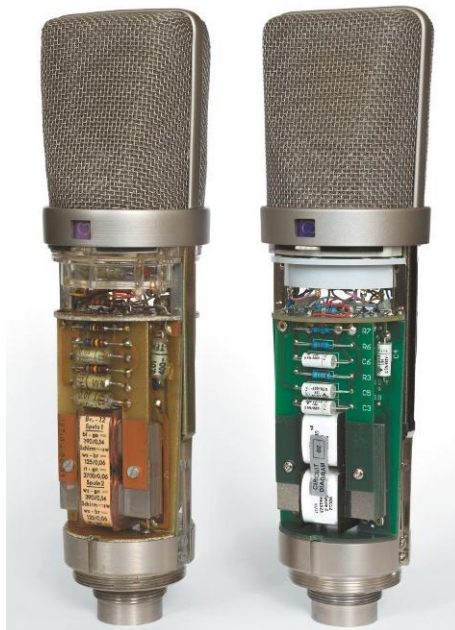
Old and new U 67 compared: The electronic layout is identical; the reissue's components are current production equivalents.
