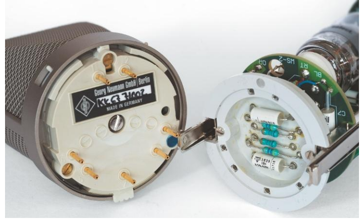
The capsule head of the U 67 reissue is based on that of the current U 87 Ai, whose materials have proven time stable.
