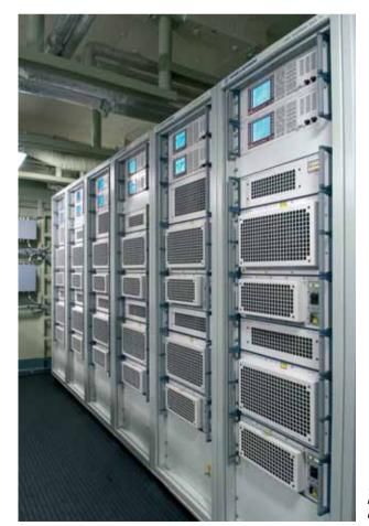
The R&S®XB2900 broadband system (in operation on a frigate)
