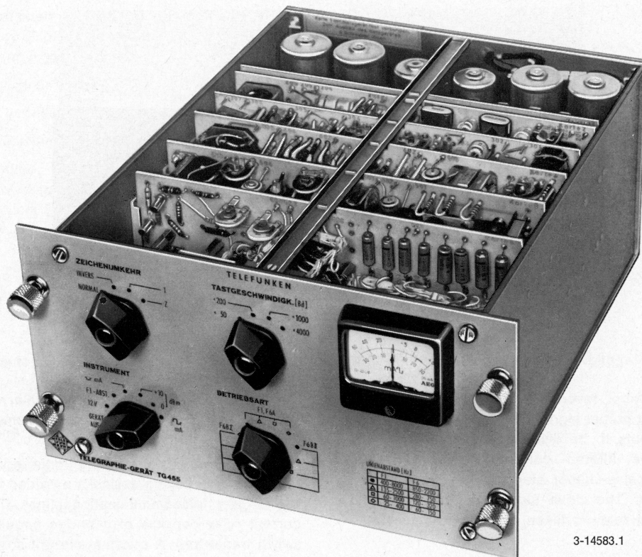
Fig. 2: Telegraphy Unit TG 455, view showing the plug-in circuit boards
